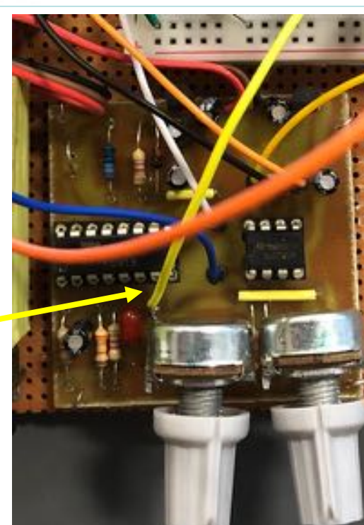
Figure 1. Function generator designed and built in Phys 310. This yellow wire enabled remote control with an Arduino.
